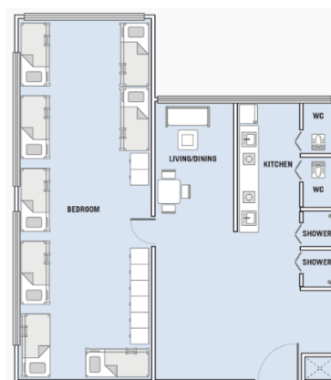
Figure 27: Current layout of Westlite Mandai with 16 workers per room, retrofitting required
